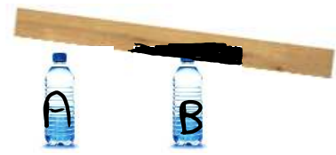
Tilted about bottle B, but plank is not falling yet, so still equilibrium
